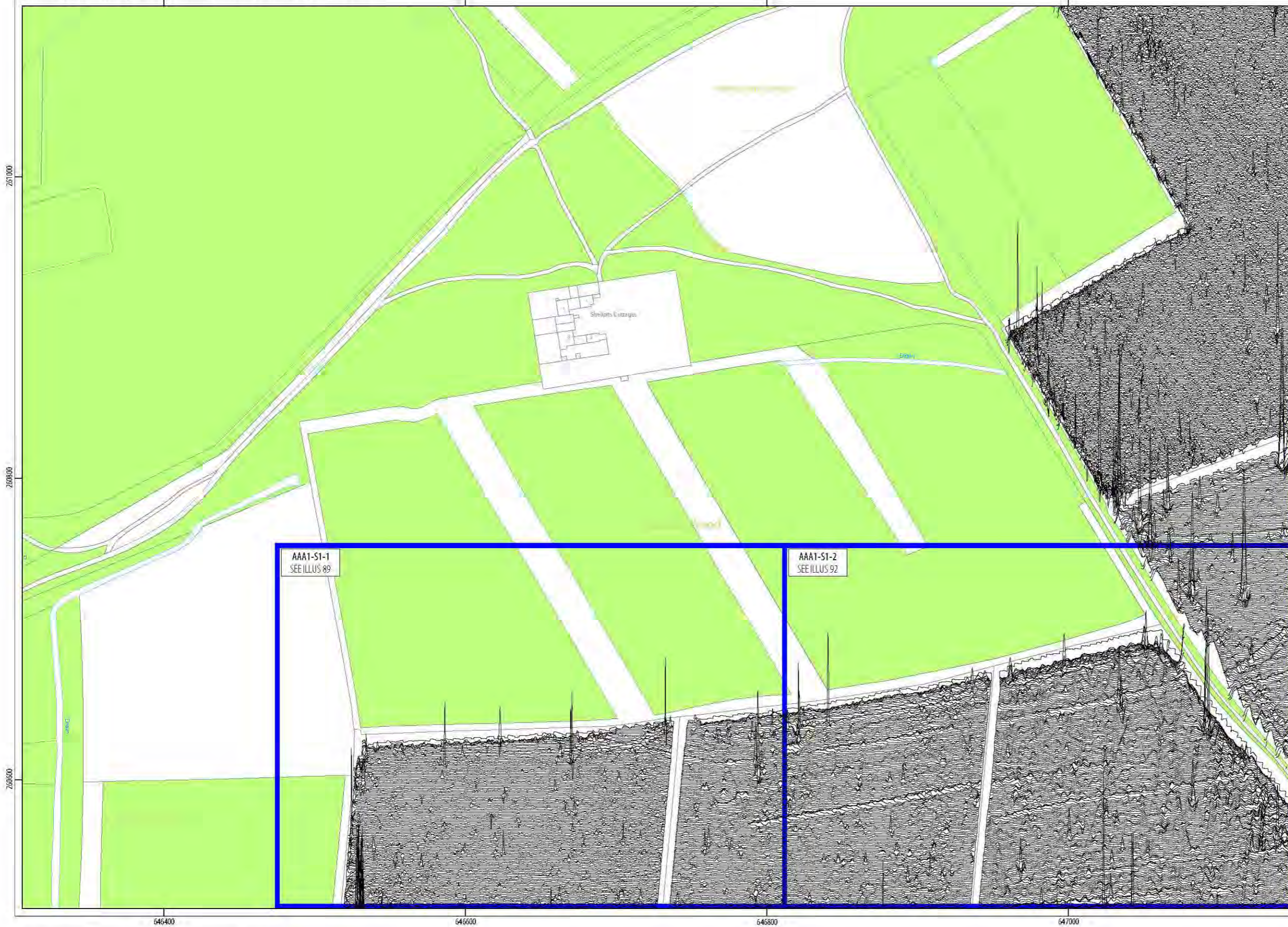
ILLUS 11 XY trace plot of minimally processed magnetometer data; Sector 1
