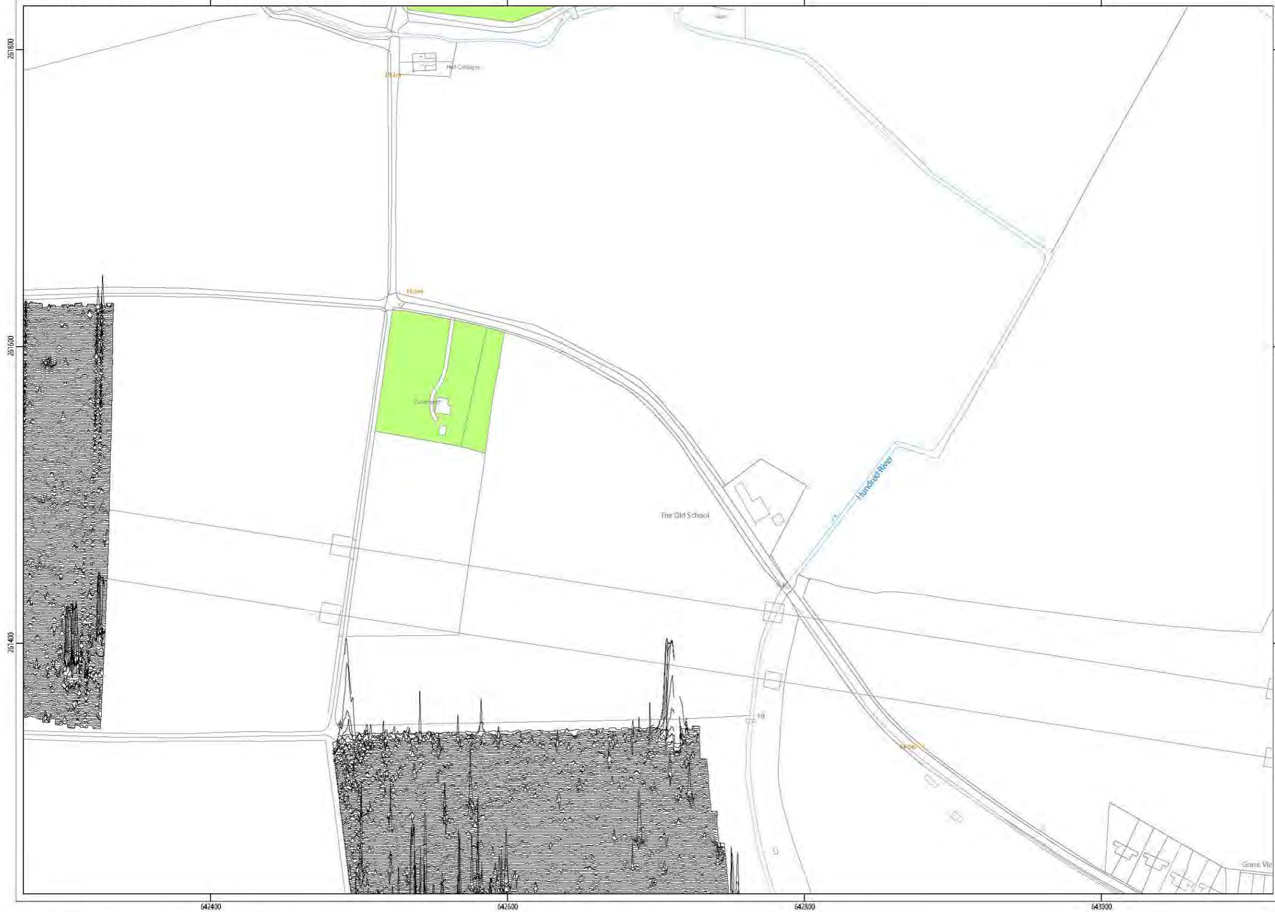
ILLUS 56 XY trace plot of minimally processed magnetometer data; Sector 16
