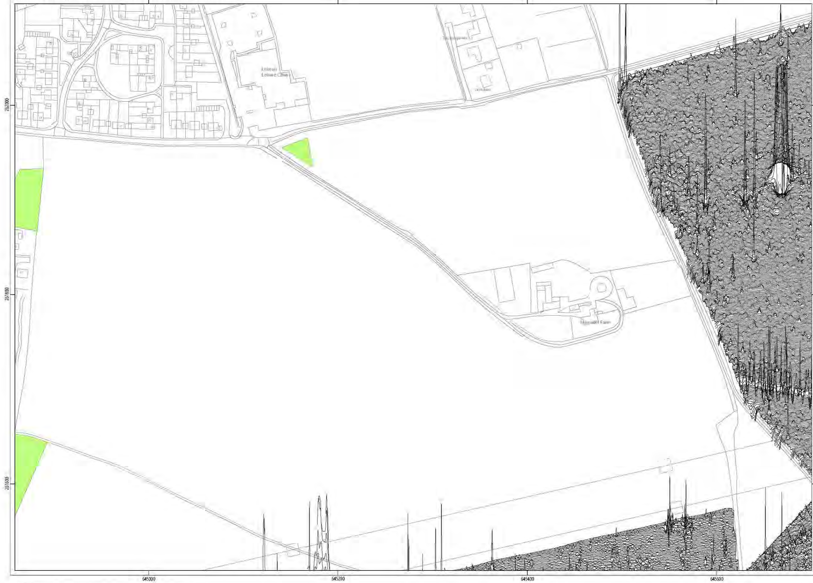
ILLUS 38 XY trace plot of minimally processed magnetometer data; Sector 10
